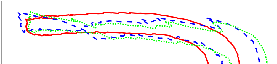
Figure 10: Plot of (the right halves of) the target 'U' shape and 'U' shapes predicted by the greedy algorithm. The solid red shape is the target 'U' shape (the shape we want to recreate from our algorithm), the blue dashed shape is the one obtained by randomly replacing any pillars, and the green dotted shape is obtained by randomly replacing the pillars that cause the largest change in distance. The discrete Fréchet distance between the blue dashed shape and the red solid shape is 0.0514 whereas the distance from the green dotted shape to the red solid shape is 0.0704.
